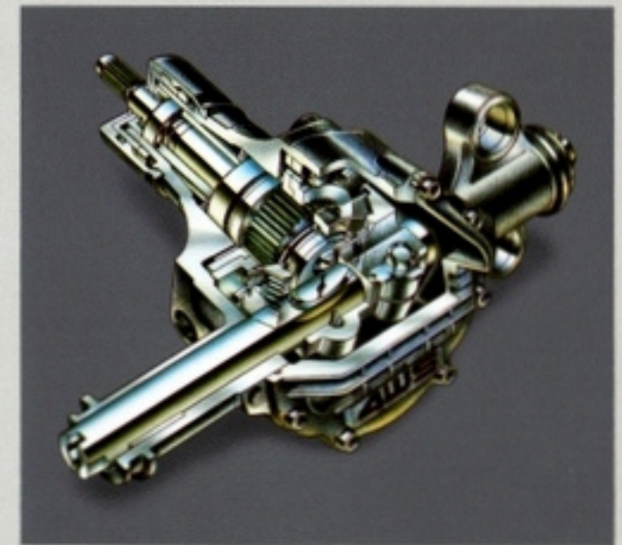
Unique, all-mechanical rear wheel steering box.
